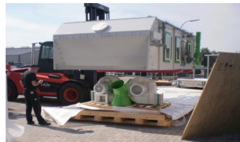
Sea worthy packaging of a waste sorter for sea transport to USA
